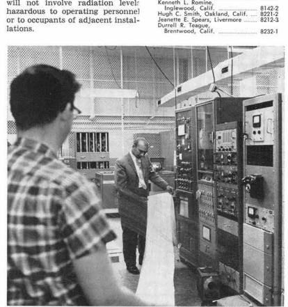
TEST DATA read out is performed after tape recording is converted to graph display in the Bldg. 860 Data Center. At left is Bob Tomlinson, operator. Marcel Reynolds is studying the test results.
